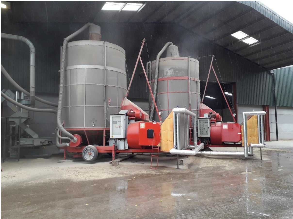
Figure 3: A pair of batch dryers in situ. Note that although these models are portable, here they have been installed permanently with augers to empty and fill the dryers, they have also been modified with hot water to air heat exchangers to supplement the heat supplied by the conventional oil burners.
