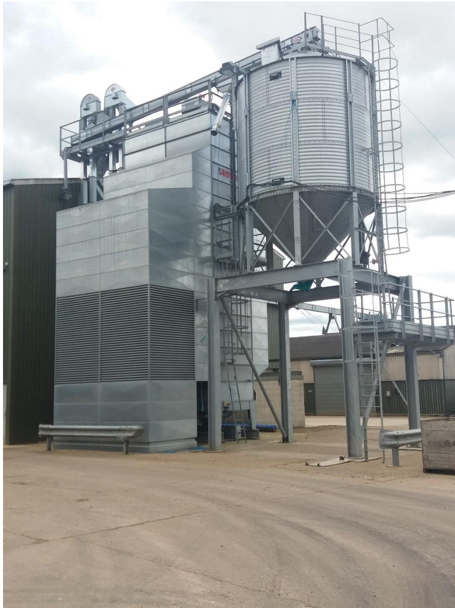
Figure 2: A continuous flow grain dryer. Note, the central tower is the dryer, the side closest to the camera is the inlet manifold, the silo to the right of the dryer is for loading grain lorries and is not directly related to drying.
